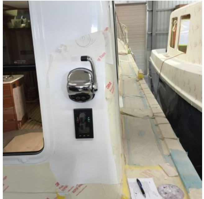
Engine and thruster controls mounted in the cockpit starboard fwd bulkhead. Very nice for docking the boat in tight spots.
