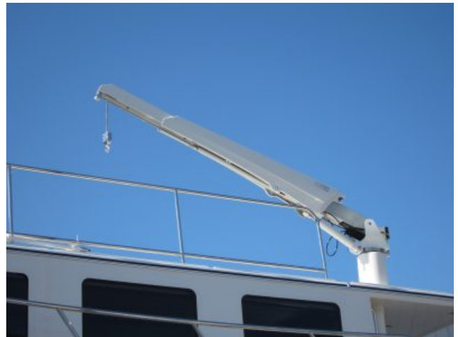
1000lb crane to get the dinghy up and down from the upper deck.
