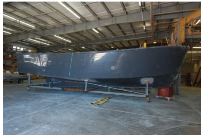
See the blue line down the hull side? That's where they are going to cut this thing in two.
