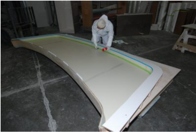
We extended our swim step to 48" so they had to make a custom mould seen here in the picture.
