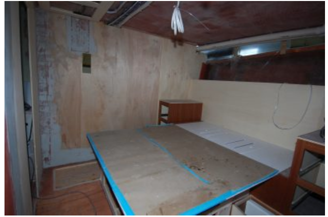
Here is the start of the master stateroom. You can see the bead platform, nightstands and the aft bulkhead.
