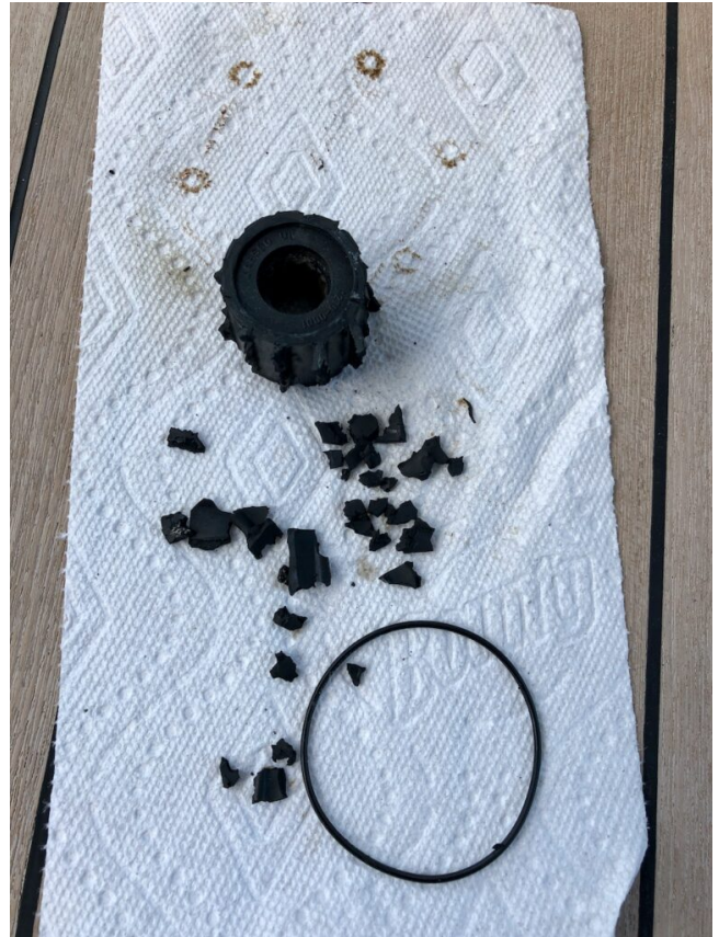
Destroyed generator impeller
